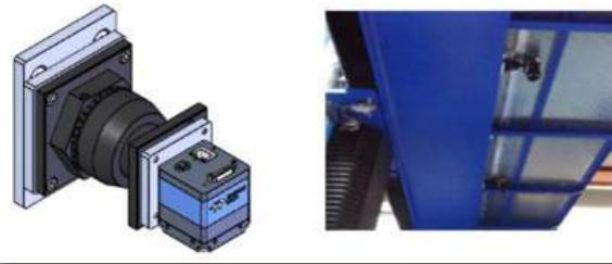
Figure 7. 2D vision cameras for base plate identification arranged on the cell portal.
