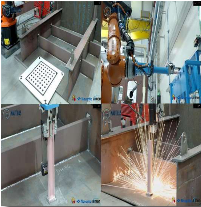
Figure 20. Different phases of the bracket assembly and welding process.
