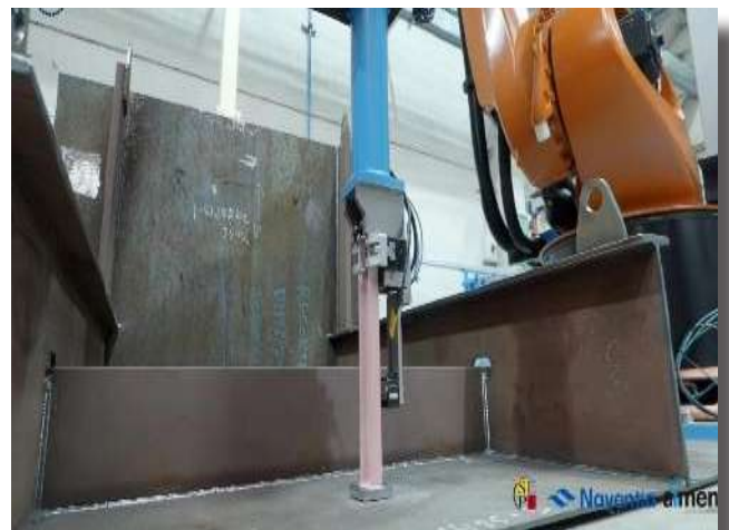
Figure 16. KUKA KR240 r3330 placement robot and handling claw.
