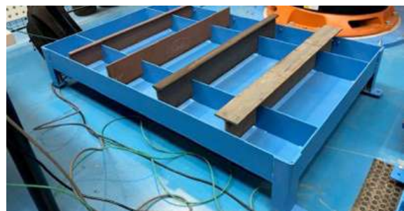
Figure 4. Basket for the accommodation of reinforcements.
