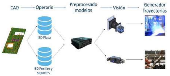
Figure 5. Schematic representation of the operation of the automated reinforcement placement and tack welding system.
