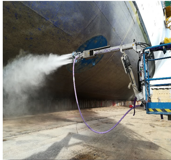
FALCH multiworker system being used in the fender of a holiday cruiser
