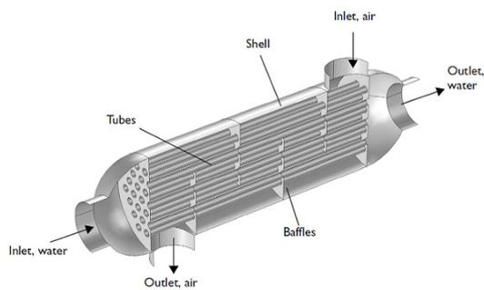
Figure 6.- 1-1 Shell and tube heat exchanger (1-Shell -1Tube pass) [5].
