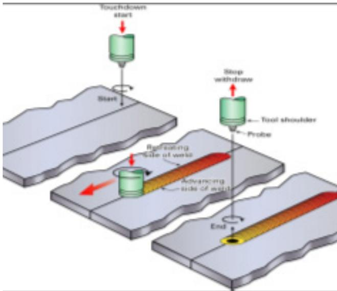
Figure 1. The general principle of friction stir welding.
