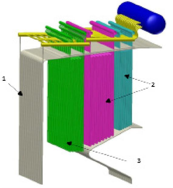
Figure 1.- Heat exchangers in a steam generator with predominance of transfer by radiation (1), convection (2), convection-radiation (3) [1].
