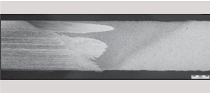
Figure 9. Metallographic section through a weld made between 8mm thick S355 carbon steel and S32205 Duplex stainless steel.
