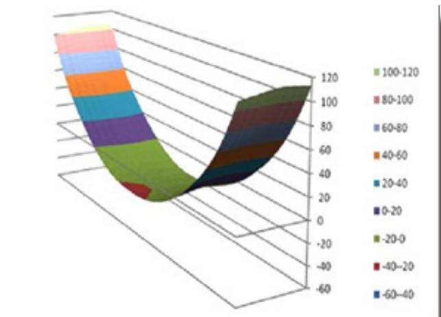
Figure 8a (above) showing the distortion measured in a SAW and 8b (below) showing the distortion in a FSW, both in 6mm thick DH36 steel. (Data courtesy of BAE Surface Fleet)
