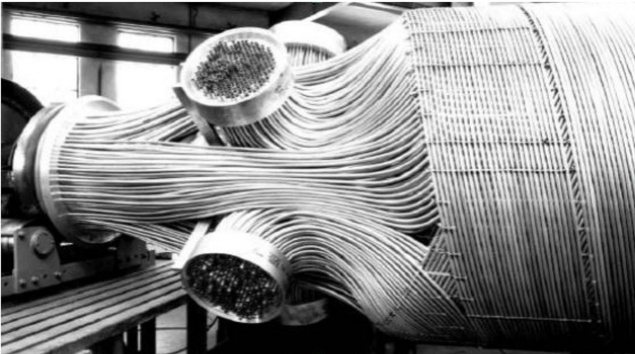
Figure 9. Linde spiral tube heat exchanger for LNG reliquefaction [7].
