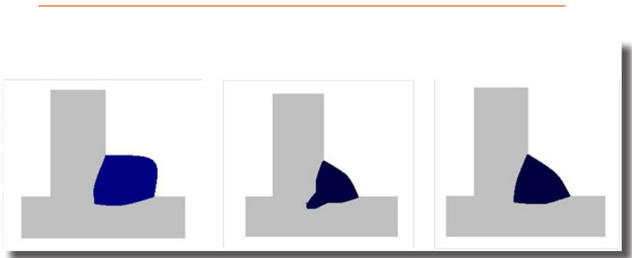
Figure: effect of CO<sub>2</sub>, argon and Ar/CO<sub>2</sub> mixtures on the penetration profile for MAG welding.
