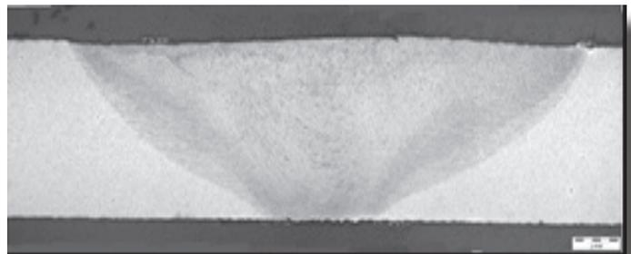
Figure 2. A metallographic section through a single pass FSW in 6mm thick DH36 steel.
