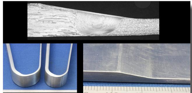
Figure 5 Example of a joint made between 4mm and 2 mm thick AA6082 sheet. The macrograph (upper) shows the weld to be defect free and the root and face bend test samples (lower left) attest to its mechanical integrity. The smooth transition between the two different thicknesses of material is shown lower right.
