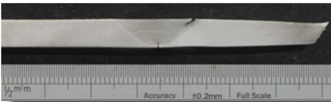
Figure 7. A metallographic section through a deliberately defective FSW in 6mm thick DH36 steel. The failure site is in the parent metal to the right hand side of the sample.
