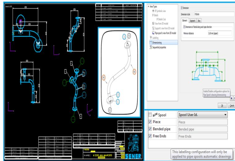
Figure 4: New area in drawings template allows to configure dimensions needed in that area of automatic drawing.
