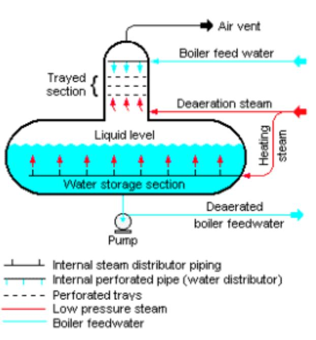
Figure 3.- Mixing or open exchanger. Application as a tray degasser [2].
