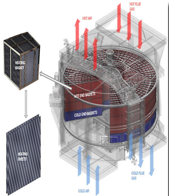
Figure 4.- Regenerative heat exchanger with rotation of the exchange surface [3].
