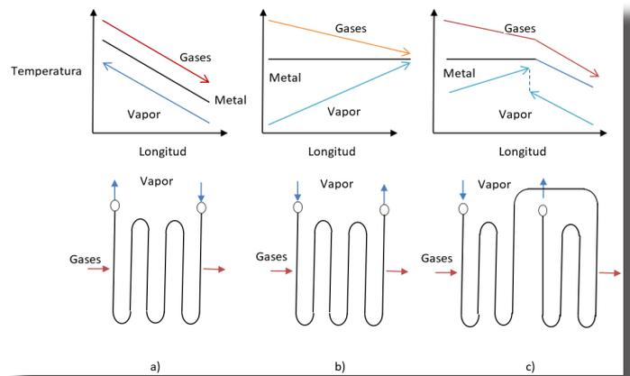
Figure 2. Temperature variation of streams and exchange surface according to counterflow (a), parallel (b) and mixed (c) configurations.
