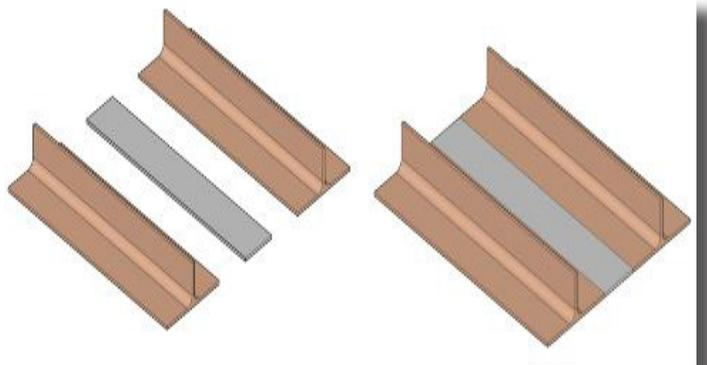
Figure 10 (above) Schematic of rolled channels and spacing plates. (Below) Example of a fully forged ISP.
