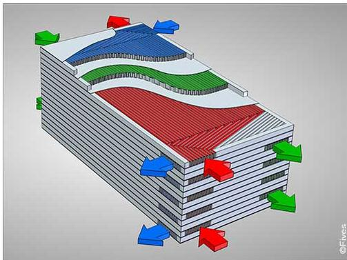
Figure 5.- Corrugated plate heat exchanger, compact, recuperative, with exchange between three streams [4].
