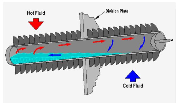
Figure 8. Thermosiphon tube where the circulation of the steam generated on the hot side, towards the cold side is represented. Once condensed, it returns by gravity to the hot side [6].
