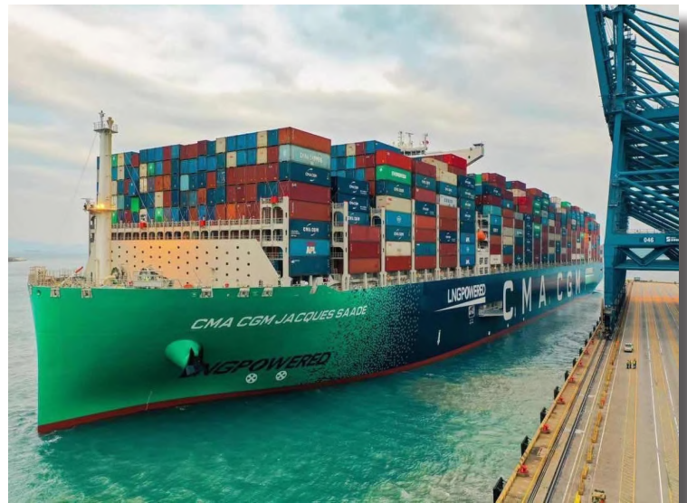
Image 1.- CMA CGM Jacques Saade containers carrier, first containers carrier in the world to be propelled by LNG.
