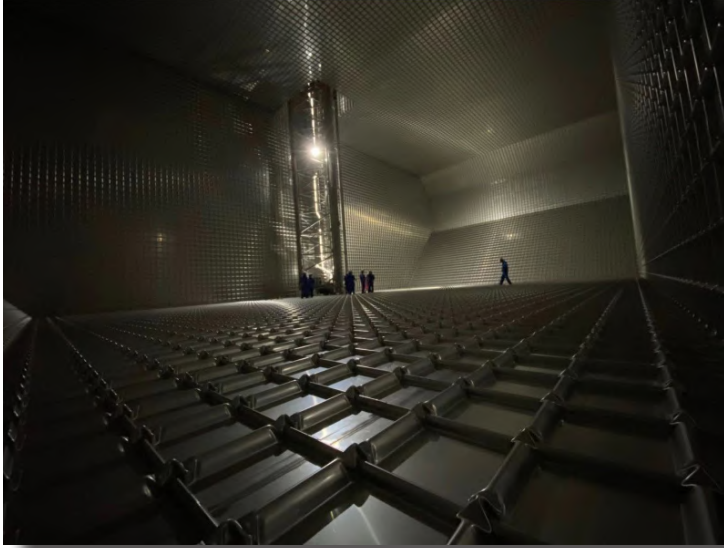
Images 5 and 6: Tank with modified design for reduction of free surfaces and conventional cargo tank (Sources: Image 5 (upper) https://gcaptain.com/chevrons-new-lng-vessels-highlighted-in-surprisingly-good-corporate-video/ , Image 6 (lower): Roland Mouron)
