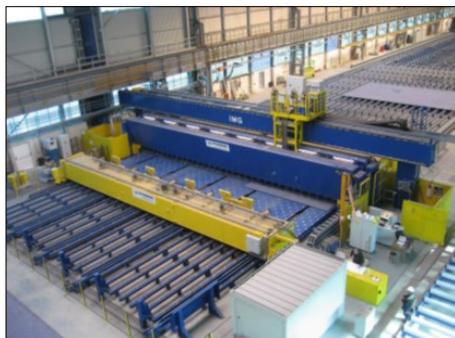
Figure 4. Installation developed by IMG for the laser-hybrid welding of cloths in the FINCANTIERI shipyard in Italy.
