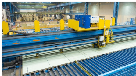
Figure 5. Laser-hybrid welding plant for reinforcements at MEYER.
