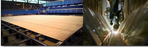
Figure 6. Installation of STX France for the welding of panels.
