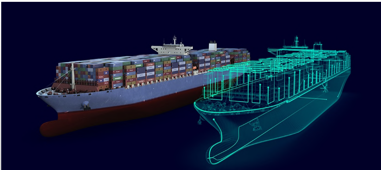
Digital twin of a vessel. Having a digital ship allows engineers to use simulation tools to understand the vessel's performance. Hydroacoustics is an area where this technology will help address the vessel's noise signature.
